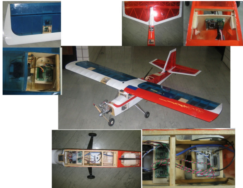
Figure 23: Demonstration UAV Showing T.I.M. Placements
