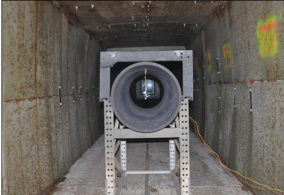
Figure 5.22 Explosive Charge within Cannon
