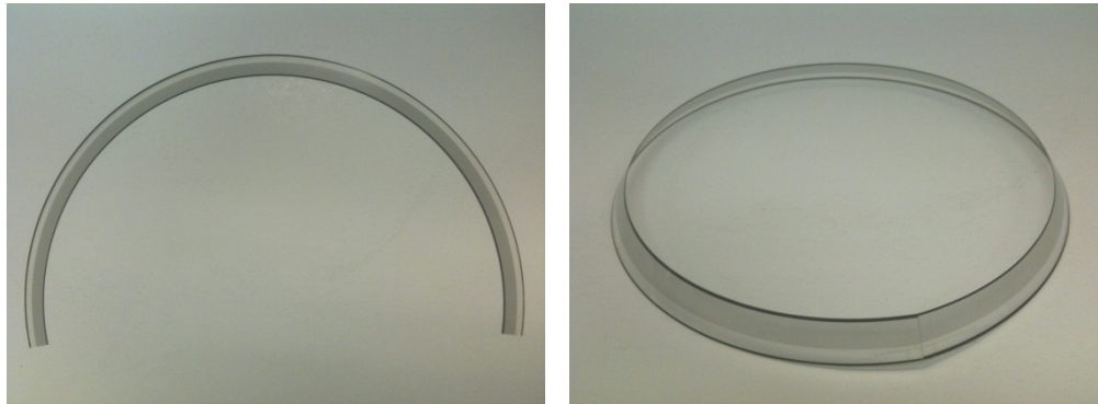
Figure 4-19. Planar image (left) used to construct the final form of the photomask (right).
