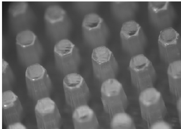
Figure 2-21 [33] . A micro-texture created on a molded seal part consists of hexagonal posts measuring 960µm tall with a 3° draft angle.
