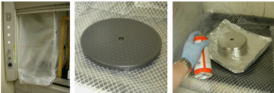
Figure 4-18. Working within a spray booth (left), a pivot platform (center) facilitated spray application (right) of Microspray™ photoresist on the conical mold insert.
