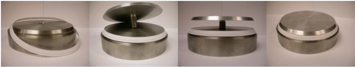
Figure 3-15. A clamp plate secures a photomask to the conical surface of a mold insert.
