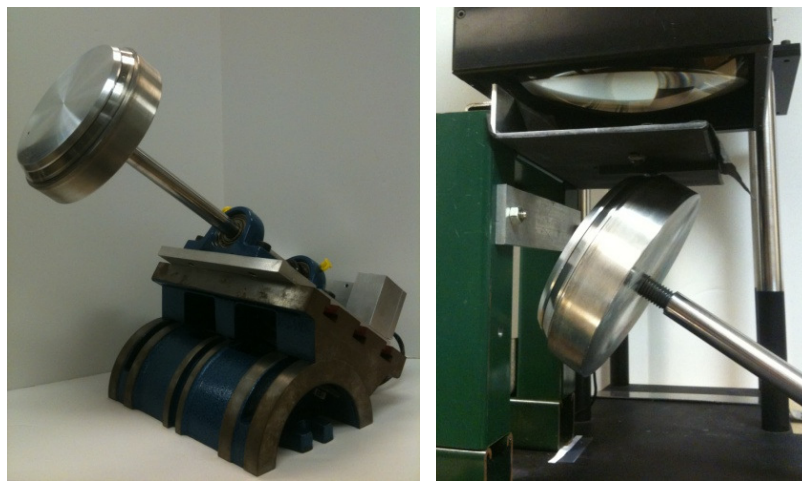
Figure 4-21. Jig developed by Impellezerri to position and rotate conical mold insert beneath ultraviolet source.
