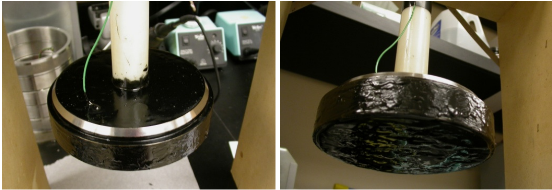
Figure 4-25. Preparations of the conical mold insert prior to electroplating.
