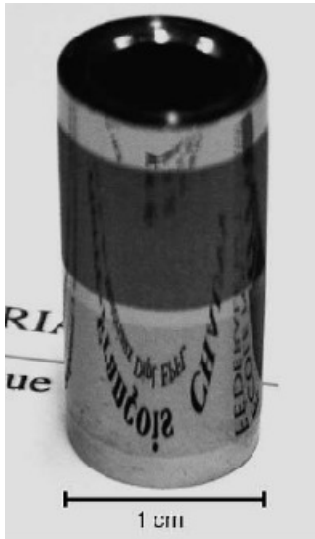
Figure 2-5 [24] . Hollow titanium cylinder covered with micro-cavities.
