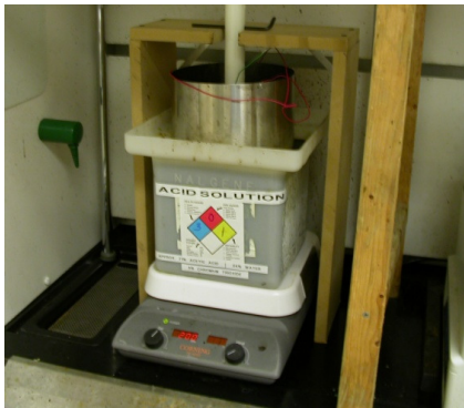
Figure 4-17. In preparation for photoresist application, the mock mold insert is submerged in an acidic solution.
