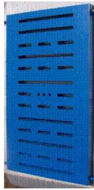
Figure 4.8: A lead sieve slit plate with a thickness of 1.5".
