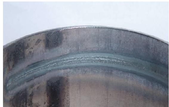
(b) Backside of the weld line
