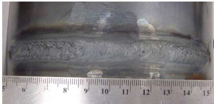
(a) Weld result (outer surface)
