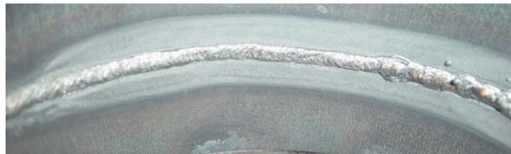
(b) Weld result (inner surface)
