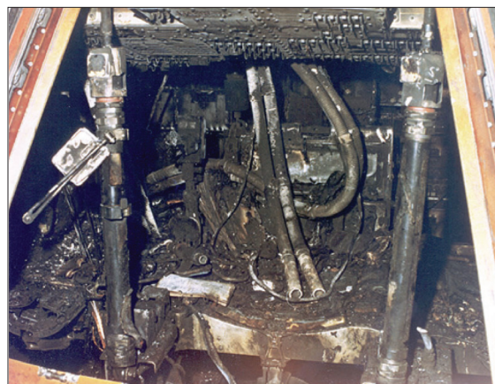
Fig. 2. The badly charred interior of the AS-204 Command Module in the aftermath of the fire. (Photo courtesy of NASA). 3
