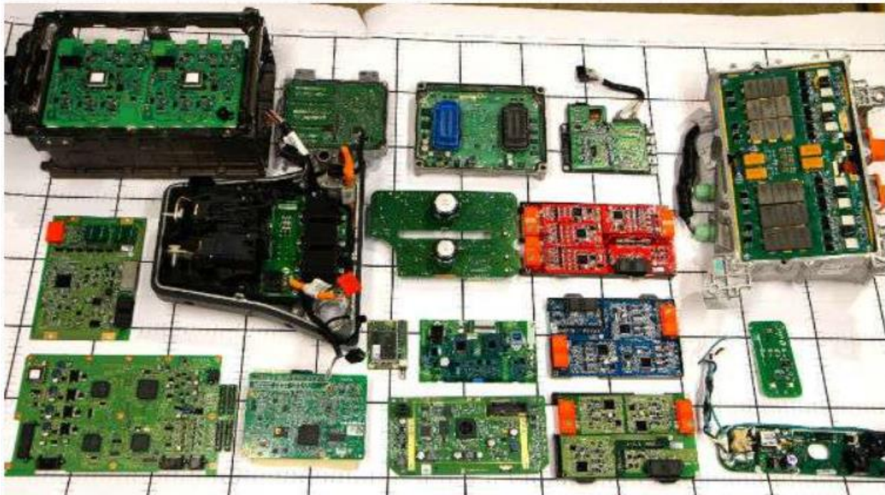
Figure 17. Chevy Volt Battery Management System
