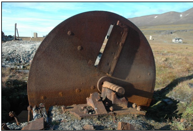
Fig 51 and 52. Remains of the rotating blubber cutter at Finneset whaling station. Right: the upper floor of the blubber cookery. Note the elevator on the far right, which transported the pieces of blubber to the first floor, and which were distributed into the cookers via a wooden distribution system. Photos: Ben Bekooy. LASHIPA 5/2007. The photo on the right has been published with the kind approval of Michigan Technological University, USA.
