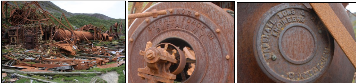
Fig 109, 110, and 111. The guano factory at Prince Olav Harbour. The guano factory contained three individual units each fitted with one heater (left), one heat fan, and one large rotating metal tube inside which the residues were processed into a fine meal. At the end of the tube, the meals were connected by a small elevator and poured into canvas bags and stored away. Left photo by G. Rossnes. LASHIPA 6/2009. Middle and right: the guano factory was designed using several manufacturers of different nationalities. The different parts were re-built and adapted on site to function as one processing unit. Photos by: U.I. Gustafsson. LASHIPA 6/2009.
