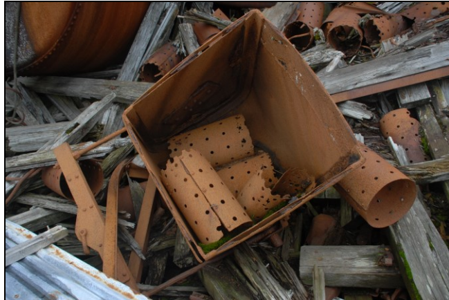
Fig 106 and 107. The internal design of a pressure cooker. The cooker was filled so that the centre grill was supported and the angled cooking grills were stacked with whale meat until the whole cooker was filled. The top was screwed solid and the steam was introduced. Right: One of the remaining bucket elevators at Prince Olav Harbour, filled with grill supports. Photo: U.I. Gustafsson. LASHIPA 6/2009.
