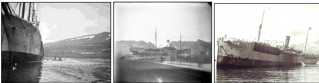
Fig 14, 15, and 16. Three steps in pelagic shipbuilding in 1905–1925; the whaling company Alfa & Betas converted the wooden sailing ship Hecla in Spitsbergen (left), a steel hulled factory ship at Deception Island, South Shetland Islands (centre), to A/S Globus and Petter Sørre's pelagic ship Lancing in 1925 (right). 159
