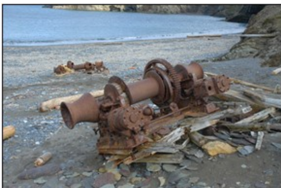
Figure 79. Feature 13. The two steam winches that were used to pull whales up for processing. The winches were produced by Pusnæs ST & MEK VERKSTED. ARENDAL. NORGE. Type No 358. Today, only the foundation for the winches remain in situ, while the winches are lying on the beach. Photo by U.I. Gustafsson. LASHIPA 5 August 2008.
