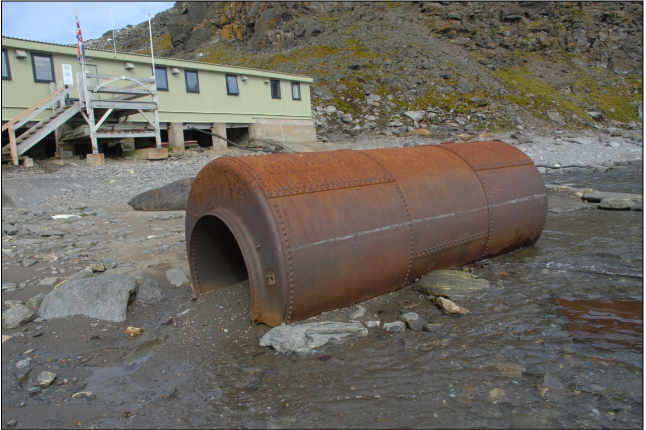
Fig 159. The steam boiler that was used at the whaling station lies on the shore in front of present day BAS research station where it is deteriorating. Photo by U.I. Gustafsson. Arctic Centre. LASHIPA 8, 2010.
