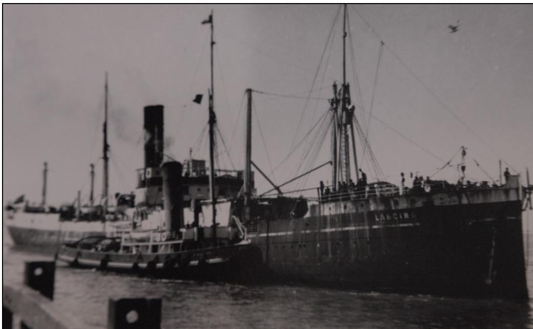
Fig 170. The factory ship Lancing. This ship was the first true pelagic factory ship that could operate independent of land. Whale carcasses could be hauled onboard and processed. 1032
