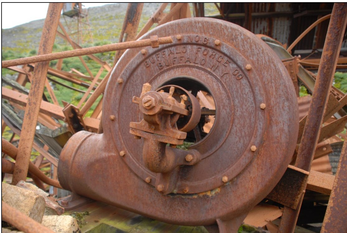
Fig 123 Left: A hot air fan produced by the American company Buffalo Forge Company in Buffalo, New York. The fan was an integrated part of the guano factory, where it was used to force large amounts of heated air into the rotating guano drier to dry the residues. Photo: U.I. Gustafsson. LASHIPA 6/2009.
