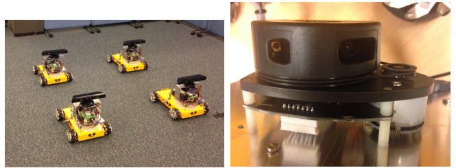
(a) The four robots employed (b) RP-LIDAR laser scanner with omnidirectional wheels. mounted at the front of each robot.
