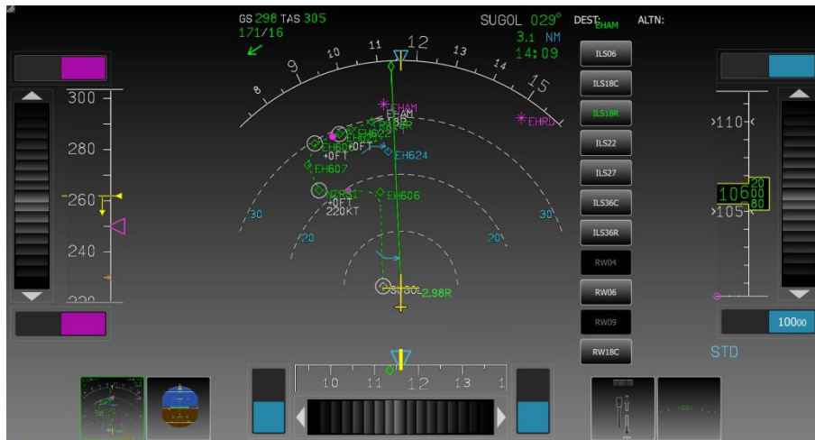
Figure 2. HMI design phase 1 using touch wheels
