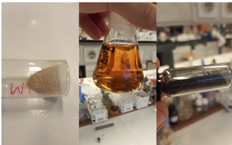
Figure S3. An aqueous solution of 1,2,4-benzenetriol (BTO), which has the appearance of a grey/beige powder (left picture), was left in time exposed to air the solution slowly darkened (middle picture), resulting in a very dark solution with a precipitate which can be isolated as a black powder after washing with water, to remove unreacted BTO, and drying (right picture)
