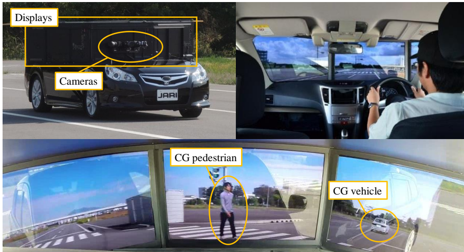
Figure 7. Augmented reality vehicle JARI-ARV (Top-left: Outer view of JARI-ARV, Top-right: Inner view of JARI-ARV, Bottom: Real front window image with superimposed CG objects).
