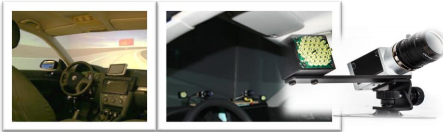
Figure 1. Driver simulator - left and eye-tracking device "Smart Eye pro" - right.
