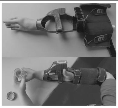
Figure 1 Prosthetic simulator.
