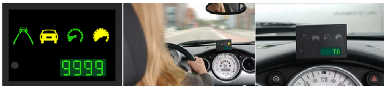
Figure 2.1 The in-car interface used in Mazureck & van Hattem (2006) to provide feedback on close following and speeding.
