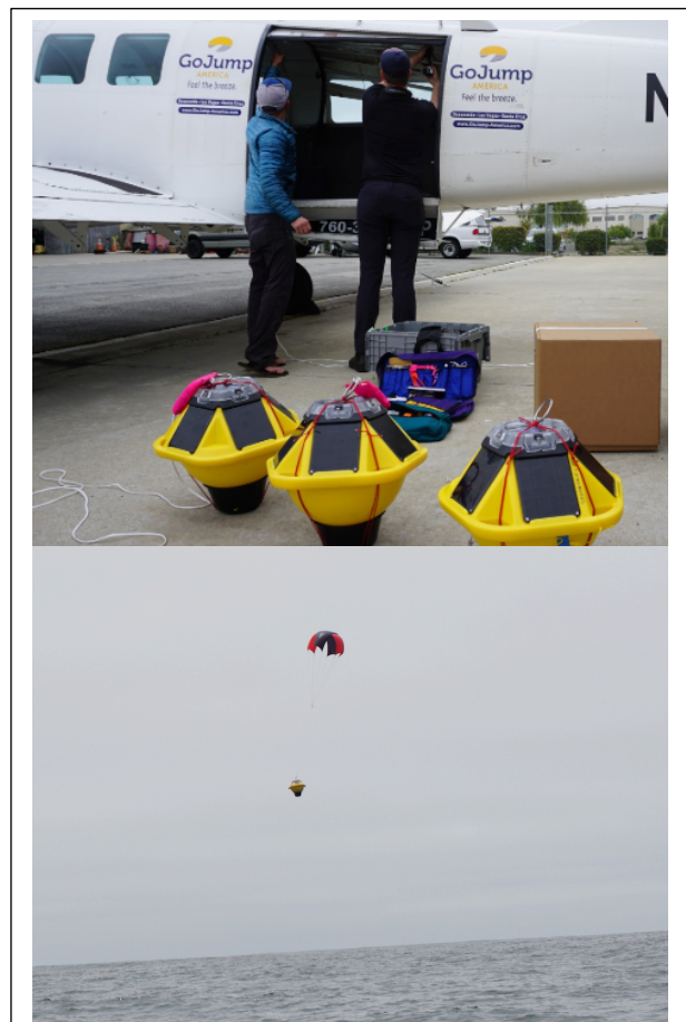
Figure 4 (top panel) Buoys being loaded into the airplane prior to deployment. (bottom panel) Spotter descending on parachute toward ocean surface near Monterey (CA, USA).
