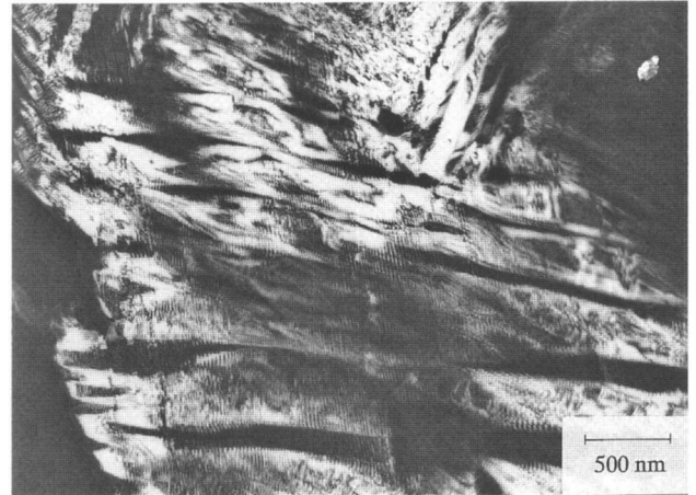
FIG. 9. Dark-field TEM image of Cr 3 O 4 on duplex SAF 2205 showing larger twins than in Cr 3 O 4 on Fe 22 wt. % Cr (Fig. 5).
