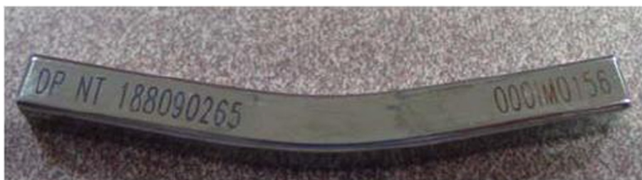
Figure 1 Square, anatomically shaped NiTi alloy spinal rod.
