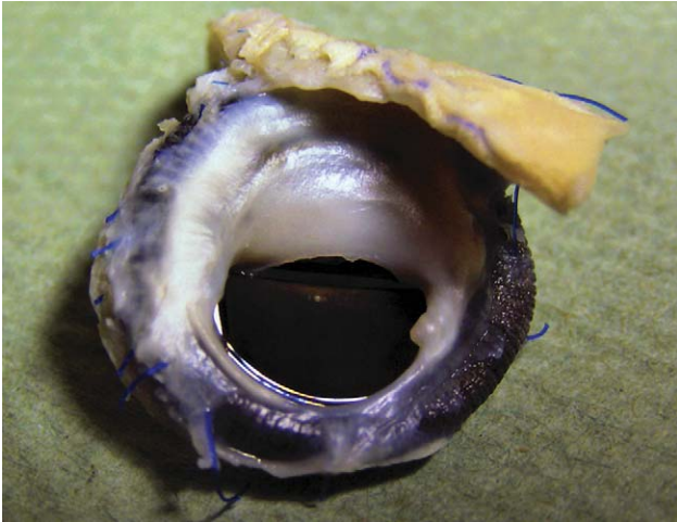
Fig. 1. Duromedics valve explanted 14 years after implantation due to valve malfunction caused by ingrowth of fibrous tissue.
