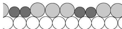
Fig. 1. Illustration of a ternary system of bigger B-particles (light gray) and smaller A-particles (dark gray) on a substrate (white) of intermediate lattice spacing. The effective misfit of the adsorbate film can be reduced by an alternating arrangement of the species.
