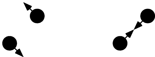
FIG. 1. Dimer rotation and dimer collision. Rotation only changes the anisotropic polarizability. Collision changes both the isotropic and the anisotropic polarizability.
