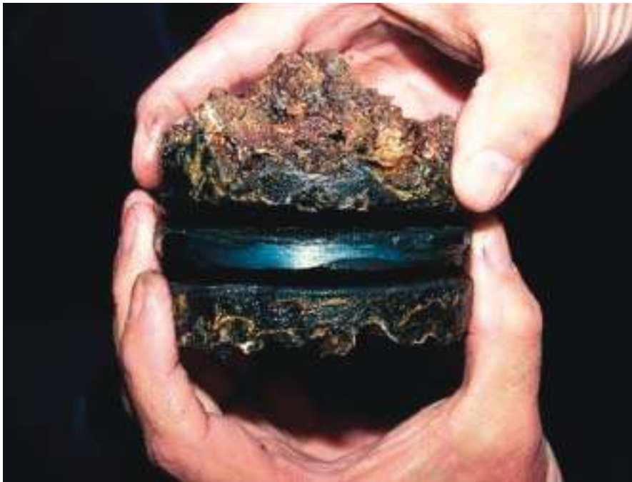
Composite interior/exterior concretion with hull metal coupon from USS Arizona ; sample taken from a water depth of 5 ft (1.5 m), port side.
