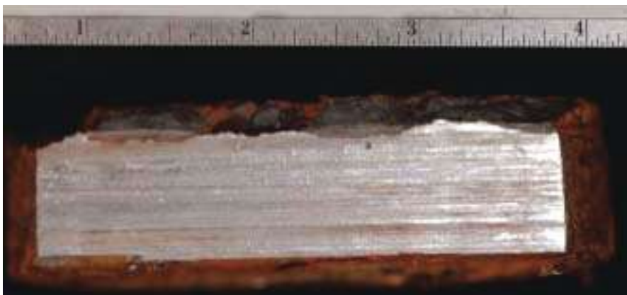
Cross section of metal coupon from USS Arizona ; sample taken from a water depth of 19.5 ft (5.9 m), port side.
