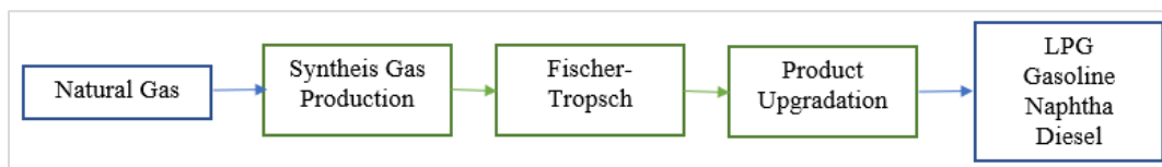
Figure 5 Block Diagram of a General GTL Process
