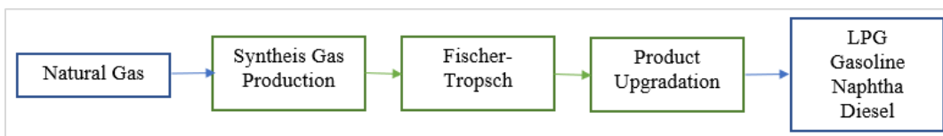
Figure 5 Block Diagram of a General GTL Process
