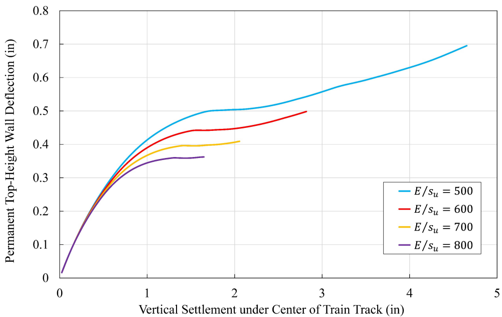
Figure 4.31. Permanent top-height lateral displacement of wall vs. vertical settlement under train track with various E/s_u ratio and 95% of full train load
