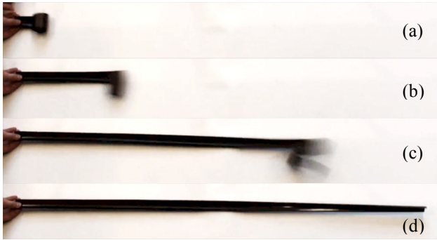
Fig. 11. Snapshots of the deployment of the tape spring. (a) t = 0.10 s, (b) t = 0.28 s, (c) t = 0.40 s, (d) t = 0.44 s.
