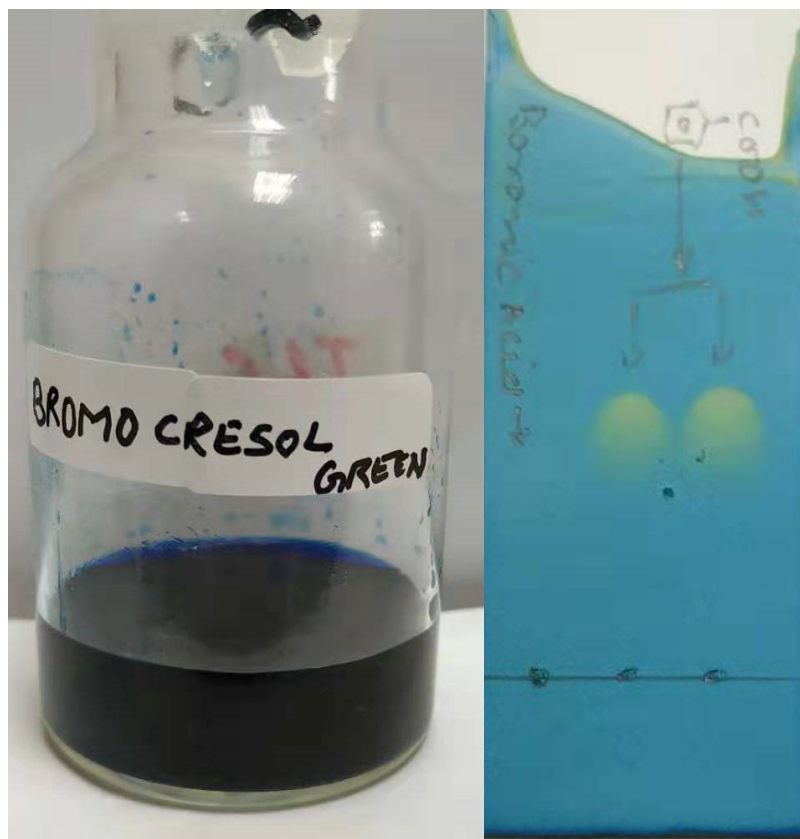
Figure S3. Bromocresol Green Solution (Left) and stained TLC with BCG for the detection of carboxylic acid (yellow spot).
