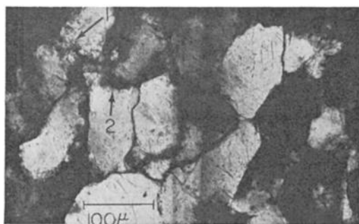
Fig. 7. Photomicrograph (crossed Nicols) showing jigsaw texture due to plastic deformation of quartz grains on a class 2 rock. Center grains have re-entrants on boundaries due to deformation. Arrows point to symplektic region (1) and to isotropic region (2) on grain boundary. The isotropic region probably contains an unresolvable mixture of coesite and diaplectic glass. Cleavages are visible on the grains. Emulsion is streaked in center of photograph.
