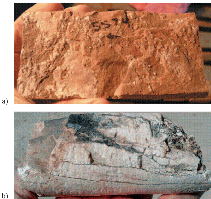
Fig. 2. Cores from Tensleep formation: a – A natural fracture face that is partially covered with crystalline dolomite, b – Highly fractured Tensleep sandstone (Lorenz & Cooper, 2004)
