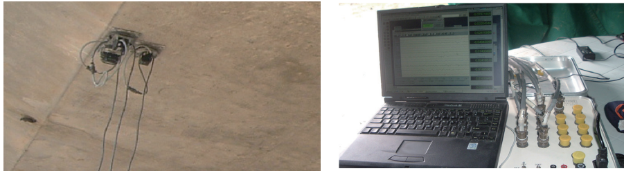
Fig. 4. Vibration sensors and data acquisition system.
