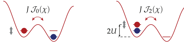
Figure 2.6.: Implementation of the gauge-field dynamics. The gauge-field particle dynamics (red) is presented for fixed positions of the matter particle (blue). In contrast to the configuration for the matter particle, an energy offset between neighboring sites of size U is introduced. This additional species-dependent tilt breaks the symmetry between the a - and the f -particles. Again looking at the effect of the energy offsets between neighboring sites taking the on-site interaction into account reveals two possible coupling processes: a zero and a two-photon transition. Here, the tunneling rate is renormalized differently depending on the two a -particle configurations but the tunneling phase is \varphi = 0 for \phi = 0 (Eq. 2.15).
