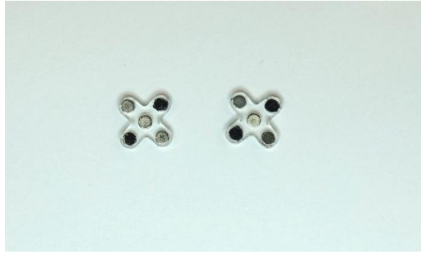
Figure 5.10 Fabricated milli-robot, the magnetic south is marked in black.
