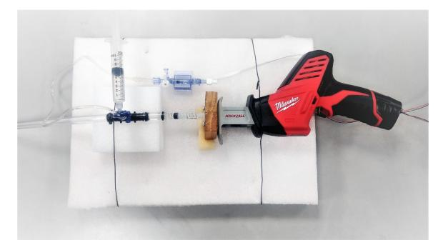
**Figure 2.5** Linear movement was generated by a battery powered reciprocating saw (Milwaukee M12 Reciprocating Saw) and transferred to the mandible via an oil filled Tygon® tubing. A pressure transducer (DPT-100, DELTRAN®) was added to the hydraulic system for measurements of the force applied by the jaw.
