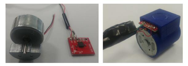
**Figure 3.1** Left: A 24 mm DC motor with eccentric rotor (JQ24-35F580C Cylindrical Vibration Motor, Jinlong Machinery & Electronics) for the application of mechanical vibrations, and the acceleration sensor (ADXL335 Triple Axis Accelerometer, Analog Devices) for recording and monitoring the displacement and frequency of the stimulations. Right: 3D printed case for covering the eccentric mass of the motor and attaching the acceleration sensor to the motor.
