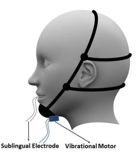
**Figure 3.2** Application of mechanical vibrations generated by an eccentric-load DC motor to the submandibular area using a chin strap.
