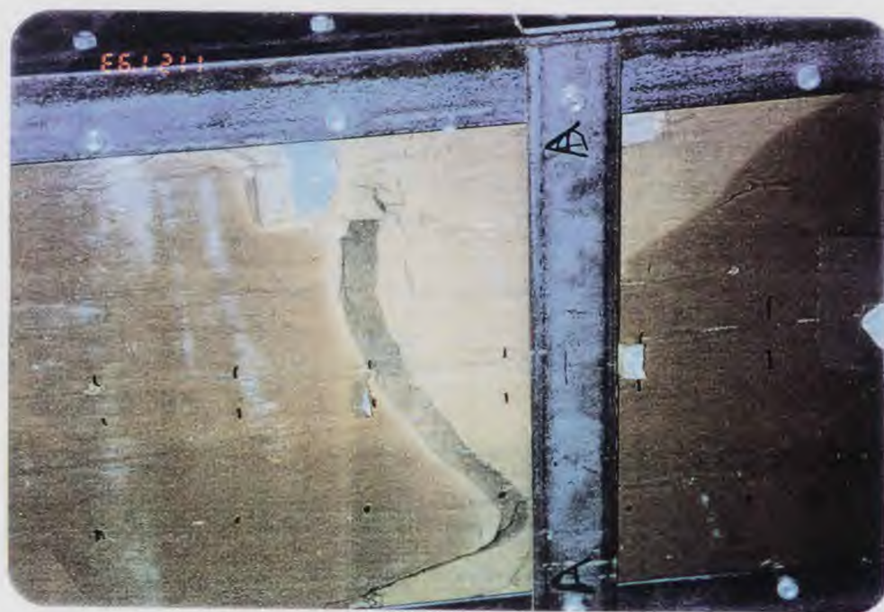
Regular Pneumatic Fracturing
