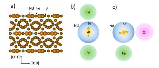
**Figure 3.2** Illustrations of atomic arrangements in the Nd<sub>2</sub>Fe<sub>14</sub>B crystal structure viewed along the [1 0 0] axis.
