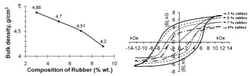
**Figure 6.5** The curve of bulk density Nd2Fe<sub>14</sub>B and BH-curve of bonded Nd<sub>2</sub>Fe<sub>14</sub>B magnet for different rubber composition
