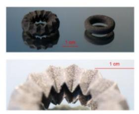
**Figure 6.1** The photograph of printed magnets of various shapes. The left object, expanded view on the bottom image, demonstrate the full power of 3D printing very complex shape, a novel functionality to the hard magnets.
