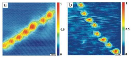
**Figure 6.20** STM image of a grain boundary on HOPG showing a 1D superlattice with a small periodicity D = 1.4 nm (a) and a large periodicity D = 4 nm (b).
