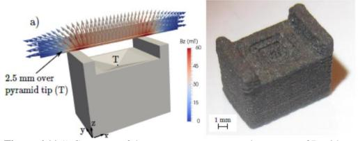
**Figure 6.11** 1) Geometry of the permanent magnet, and area scan of B with a step size of 0.1mm in the middle of the printed magnet. 2) Printed isotropic NdFeB magnet with Neofer ® 25/60p with optimized shape to suppress  $B_x$  and  $B_y$  along the x-axis  $r_x$ .
