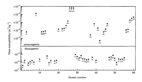
**Figure 2.7** The mass susceptibility of the first 60 elements in the periodic table at RT, plotted as a function of the atomic number. Fe, Co, and Ni possess spontaneous magnetization with applied magnetic field.
