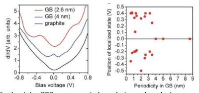
Figure 6.21 On the right, STS on two grain boundaries and on the bare graphite surface
