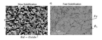
**Figure 6.3** SEM picture of the printed sample with slow solidification on the left and fast solidification on the right side.
