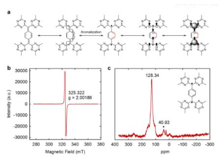
**Figure 6.16** (a) Schematic representation of the radical formation and its stability in the structure.; (b) solid-state ESR spectrum of the sample under ambient conditions, showing an isotropic singlet; and (c) solid-state NMR revealing the presence of an unusual peak at 40.93 ppm, which is associated with the tertiary radical in the structure (indicated in the inset by a black dot).
