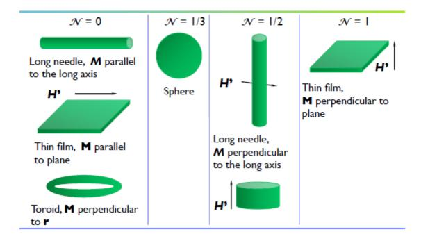
**Figure 2.1** Demagnetizing Shape Factors.
