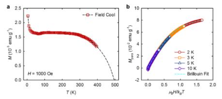
**Figure 6.24** Magnetization as a function of the temperature, recorded at 1000 Oe. Robust spontaneous magnetization persists up to 400 K. The estimated critical temperature is Tc  $\sim$  495 K (b) magnetization as a function of  $\mu_B H/kBT$  at various temperatures
