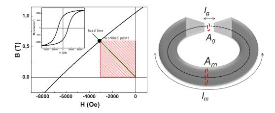
**Figure 2.9** a) Plot of the 2nd quadrant of the B-H hysteresis loop. The shaded area represents the maximum energy product, (BH)<sub>max</sub> b) Depiction of the open magnetic circuit comprised of a permanent ring magnet, two soft magnetic ends to guide the magnetic flux and an empty airgap
