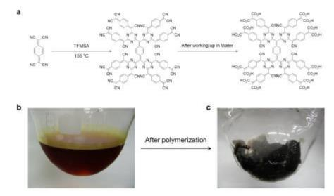
**Figure 6.12** (a) Illustration of TCNQ framework with edge groups after aqueous quenching; (b) TCNQ dissolved in TFMSA after stirring at room temperature before self-polymerization; (c) complete gelation of the reaction mixture after polymerization at 155 °C overnight.
