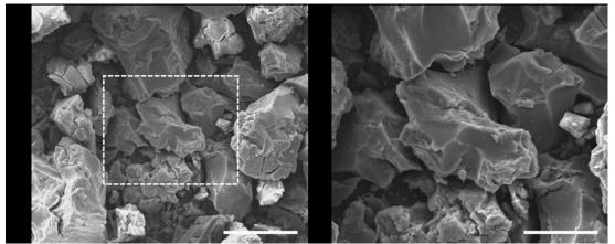
**Figure 6.14** SEM images of the p-TCNQ at different magnification showing compact and irregular morphology: a) resolution scale of  $100~\mu m$  b) Higher resolution scale of  $50~\mu m$
