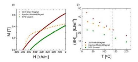
**Figure 6.4** a) Magnetization as the function of demagnetizing field for three different samples, all based on the same MQP – S powder: 3D printed, Injected molded magnet with most used PA 12 polymer, and SPS sintered. b) Temperature dependence of the (BH)max for the same three samples.
