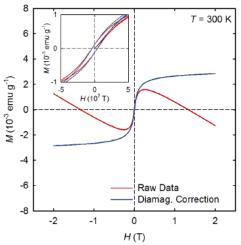
**Figure 6.22** Magnetization as a function of field recorded at 300 K. Dark red line represent the raw experimental data of magnetization. Dark blue line represents the magnetization after subtracting linear diamagnetic background.
