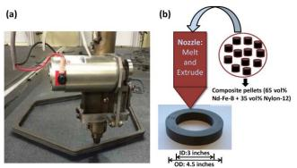
**Figure 6.7** (a) Image of the nozzle depositing layers of magnetic materials on the print bed; (b) Schematic of the melt and extrude process, right underneath the nozzle is a printed magnet in a hollow cylinder shape.
