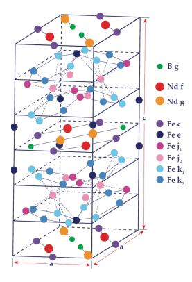
**Figure 3.3** Unit Cell of Nd<sub>2</sub>Fe<sub>14</sub>B. The c/a ratio exaggerated to emphasize the puckering of the hexagonal iron nets.
