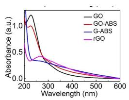
**Figure 6.30** UV-vis spectra of separated samples dispersed in aqueous solutions, including GO, GO-ABS, G-ABS, rGO.
