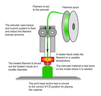
**Figure 2.17** Basic FDM Setup.
