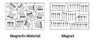
**Figure 2.8** Domains not aligned to the left; Domains aligned due to magnetizing force Source: Garrett, Casey."Caseygarrettphysics". Caseygarrettphysics.Blogspot.Com, 2018, http://caseygarrettphysics.blogspot.com.
