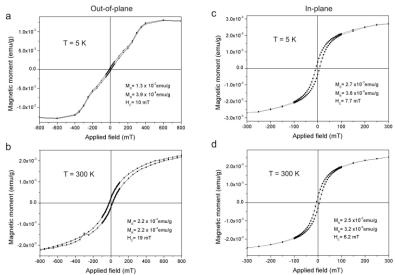
**Figure 6.26** Out-of plane (a,b) and in-plane (c,d) SQUID magnetization measurements on HOPG after subtraction of the diamagnetic signals at 5 K and 300 K. Magnetic field has been applied along the c axis in the out-of-plane direction and along the graphene planes in the in-plane direction.
