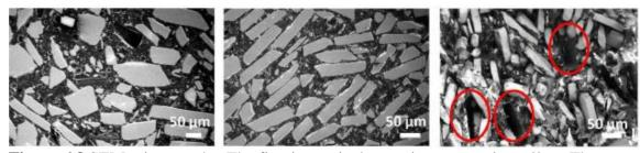
**Figure 6.8** SEM micrographs. The first image is the starting composite pellets. The second image is the BAAM printed bonded magnets. The third shows the fractured surface of the BAAM magnets after tensile testing.
