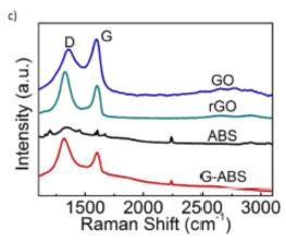
Figure 6.29 Raman spectra in prepared GO, rGO, ABS and G-ABS samples.
