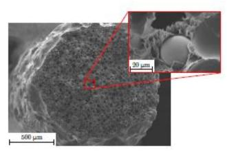
**Figure 6.10** SEM micrograph of the Neofer ® 25/60p filament, NdFeB spheres inside the PA11 matrix
