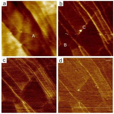
**Figure 6.19** The same area on the HOPG surface imaged with AFM (a), MFM (b) and (c), and EFM (d). MFM tip has been magnetized into the graphite surface (b) and out of the graphite surface (c), respectively
