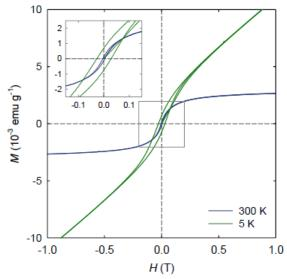
**Figure 6.23** Magnetization as a function of the applied field (H), recorded at 300 K and 5 K with the diamagnetic background subtracted from all data. The material possesses spontaneous magnetization, even at 300 K. Closer view of the hysteresis loop is shown in the inset.
