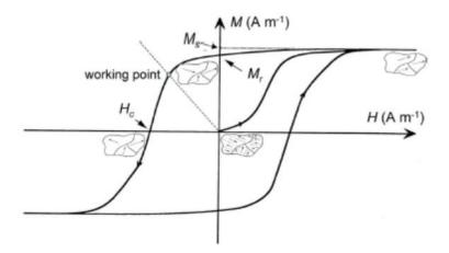
**Figure 2.5** An M(H) hysteresis loop for a hard-magnetic material, with indications of the crystallite structure and domain structure at different points around. The dotted line, with slope-1/N intersects the loop in the second quadrant at the working point of the magnet.
