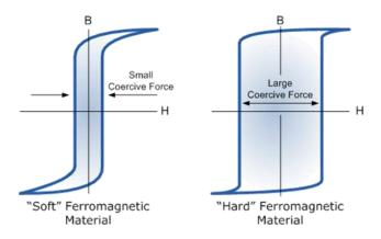
Figure 2.6 Hysteresis Loops of the Soft and Hard Ferromagnetic Materials
