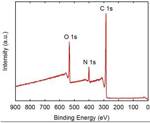
Figure 6.15 XPS survey spectrum from the p-TCNQ.
