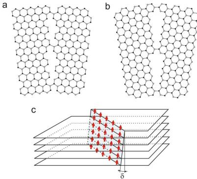
**Figure 6.27** Models of two basics shapes of grain boundaries in graphite: (a) armchair direction with periodicity D and (b) zigzag direction with periodicity 3D. (c) 2D in-plane magnetized grain boundary propagating through bulk HOPG.
