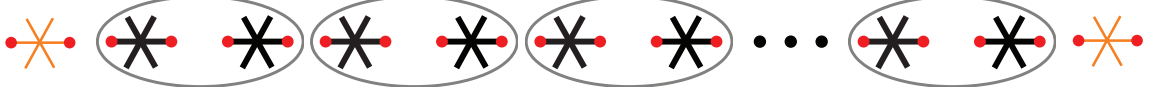
Figure 4.4 The 1D spinner system with the two fixed side spinners. Grey line demonstrated unit cells.
