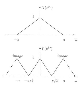
Figure 4.4 Frequency domain representation of the Upsampling by 2, with the input signal (top) and the upsampled signal (bottom).
