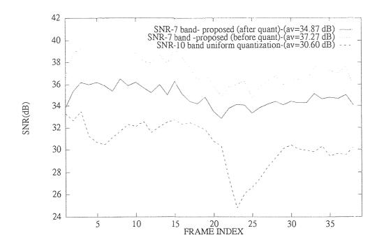
Figure 6.2 Frame by frame variation of the average  $SNR_{pp}$  values in dB for the test sequence "CINDY".
