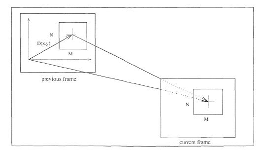
Figure 2.2 Block matching motion estimation
