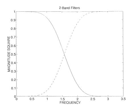
Figure 6.1 Frequency responses of the 8 tap separable low-pass and high-pass filters. seen from the figure, modeling brings some error, but this error can be tolerated for the low bit-rate coding applications.
