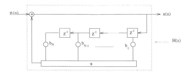
Figure 3.1 Filter Model of AR(N) Process
