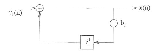
Figure 3.2 Filter Model of AR(1) Process
