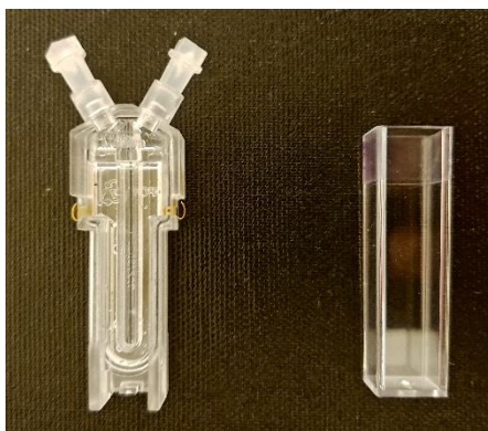
Figure 5.3 Folded capillary zeta cell (model DTS1070) and 12mm square polystyrene cuvettes.
