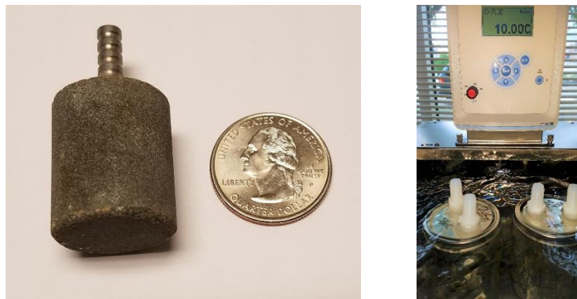
Figure 3.19 Diffuser used in ozonation and the constant temperature bath.
