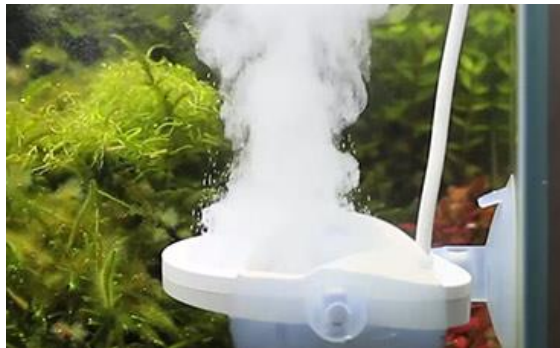
Figure 3.6 Electrolysis bubble generation in fish tank.
