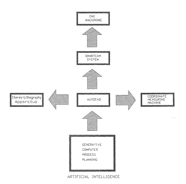
Figure 11. Linking Thesis Software to other Manufacturing Functions
