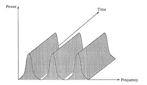
Figure 2.1 FDMA channelization
