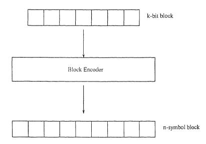
Figure 2.9 The fundamentals of block coding.
