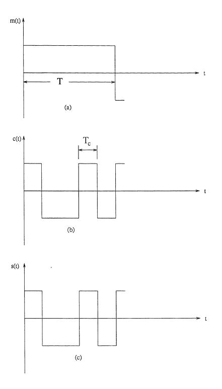
Figure 1.1 Signal waveforms in a spread spectrum system. (a) The original data sequence, m(t). (b) The spreading sequence, c(t). (c) The spread spectrum signal, s(t) = m(t)c(t). The processing gain N = 5.
