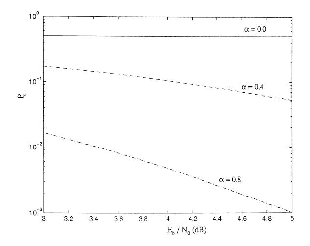
Figure 3.5 Error performance of the desired user with differing levels of path-loss (soft-decision decoding)
