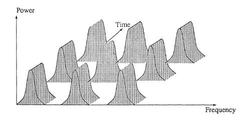
Figure 2.2 TDMA channelization
