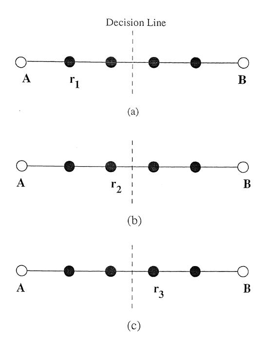
Figure 2.12 The concept of free distance
