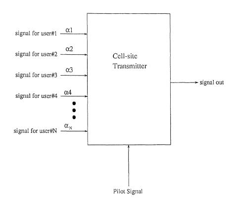
Figure 2.7 Generic CDMA cell-site transmitter/receiver structure. The constants  $\alpha_1, \ldots, \alpha_N$  are scaling constants used for power control purposes.
