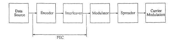
Figure 2.6 Generic CDMA mobile terminal modem structure
