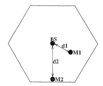
Figure 2.5 An example single-cell configuration used to discuss the problems of multiple access interference and near-far effect in cellular CDMA
