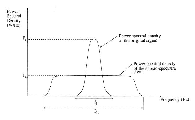
Figure 1.2 Power spectral density plots showing the effect of spread spectrum modulation on a signal.
