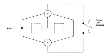
Figure 2.10 A 4-state convolutional encoder
