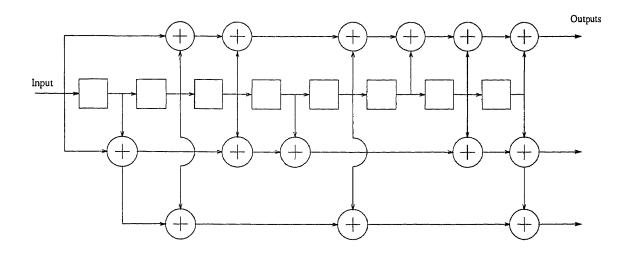
Figure 2.11 A 256-state convolutional encoder
