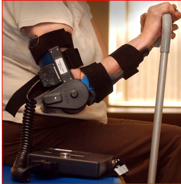
Figure 1.2 The Myomo e100 neuromotoric device incorporates EMG technology to improve elbow motion after stroke. After bicep or tricep surface electrodes detect even trace muscle contraction, a motor in the device assists with the individual's desired movement [39].
