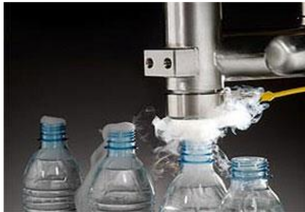
Figure 4.1 Example of Nitro Dozer
