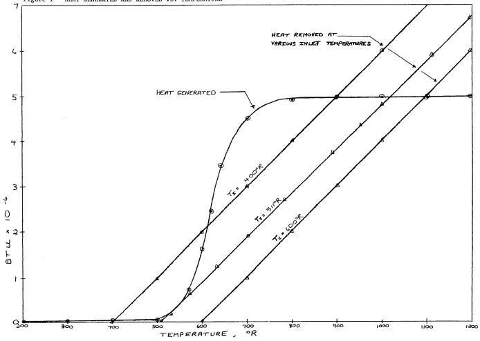
Figure 1 HEAT GENERATED AND REMOVED VS. TEMPERATURE
