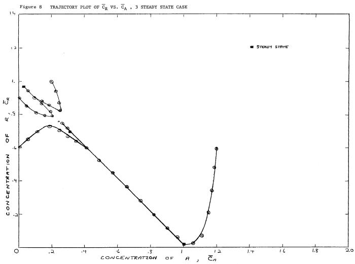
system seemed to wander about the region, in some cases falling back to the lowest steady state and in some others, becoming unstable. Any trajectory passing through or near the middle steady state as though the point was did not exist. The regions of asymptotic stability are evidently relatively small for the high steady state and relatively large for the low steady state.
