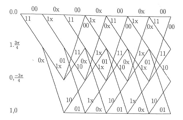
Fig. 11. Trellis diagram of [1 + D, 1, 1 + D]combined coding and TFM modulation produced by periodically deleting bits from the R = 1/2, v = 1 code [1 + D, 1].
