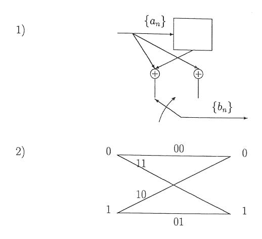
Fig. 6. Trellis coded modulation for the encoder  $$[1{\rm +D}\ ,\,1]$$
