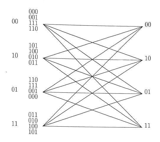
Fig. 8. Trellis diagram for the encoder in Eq. (5.2) with R = 2/3, v = 1.
