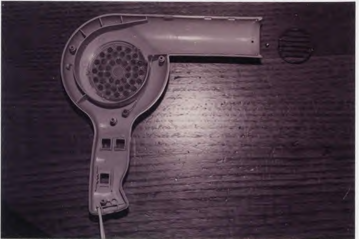
Figure 13.2 Hand Held Hair Dryer Showing the Top Shell, Fan Filters and Nozzle Vent
