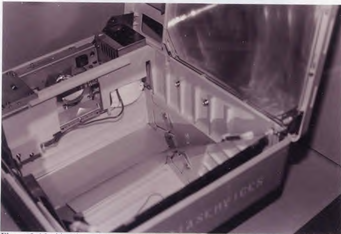
Figure 9.4 Inside View of the Projector Showing Switch, Body Lens, Hinge and Elevator
