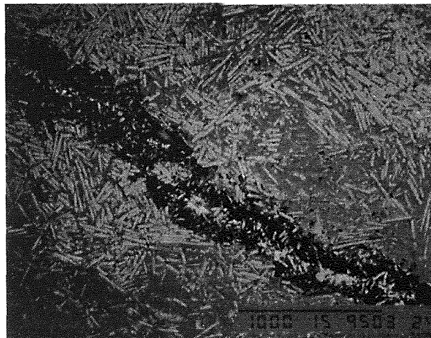
Figure 20 Random chopped fiber concentration on the tensile side surface of a 40% flexural test failed specimen (35X).
