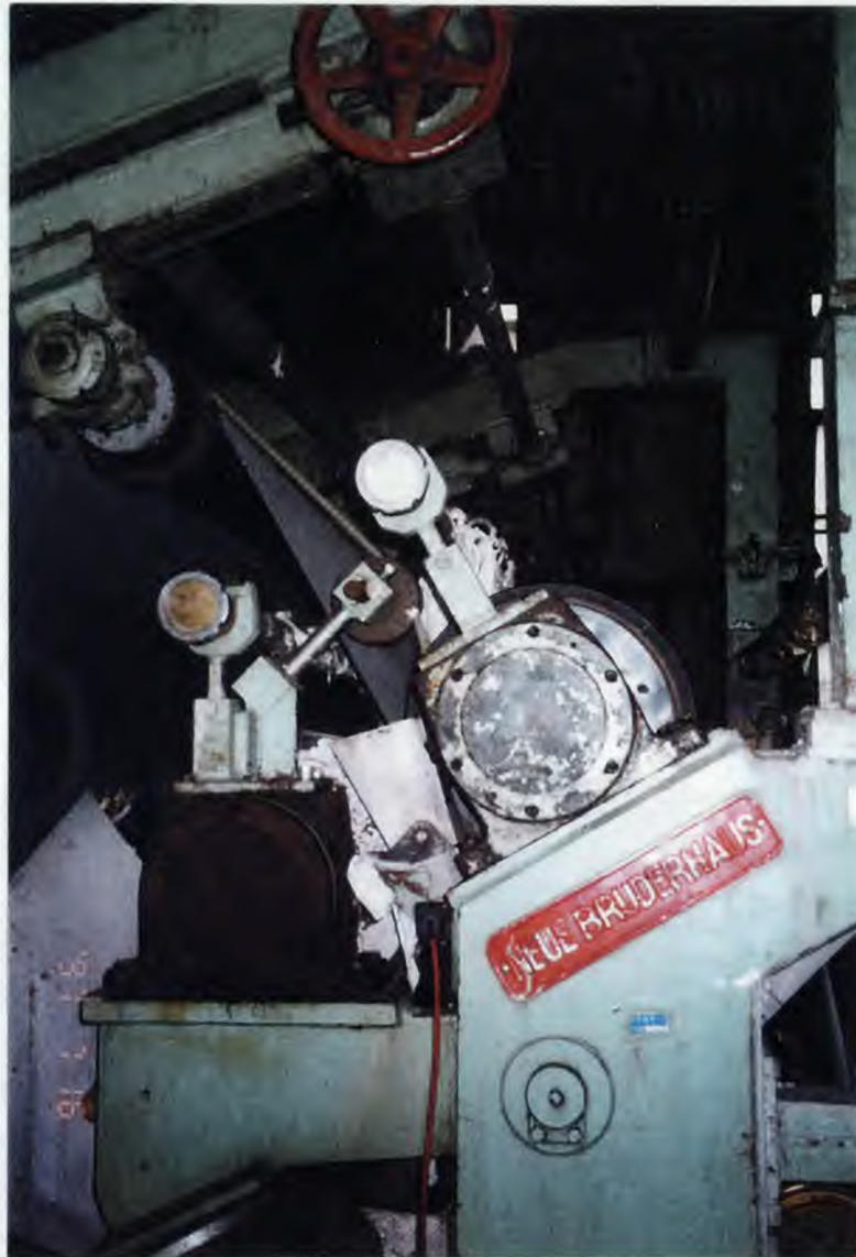
Photograph 15. The Calender Process: Press to Reduce Paper Thickness and Produce a Smoother Surface
