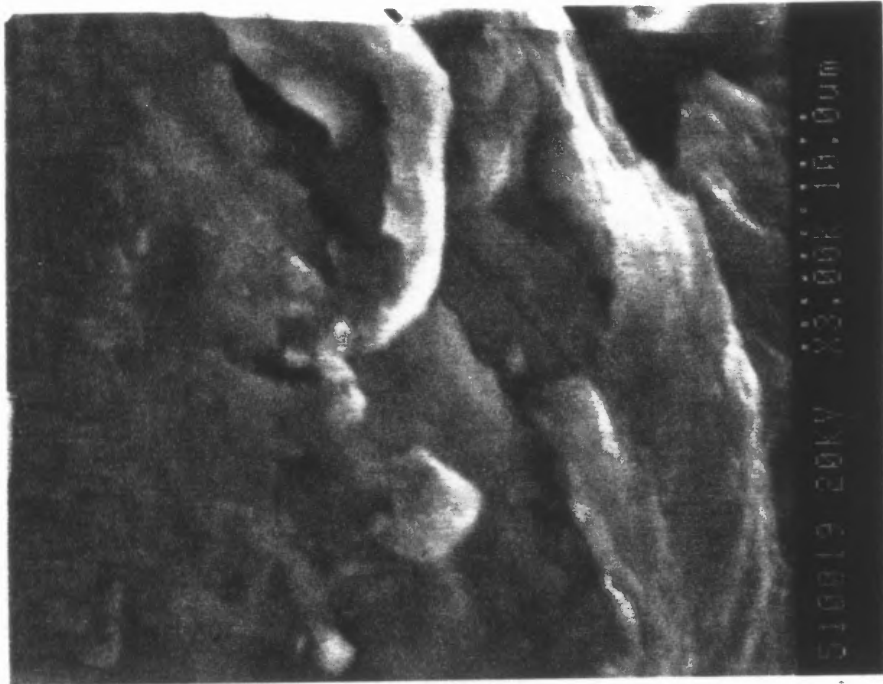
Figure 5.25. Sample 2 Aluminum plate under WJ cutting. Note: Plastic deformation in the edge of the flat surface.
