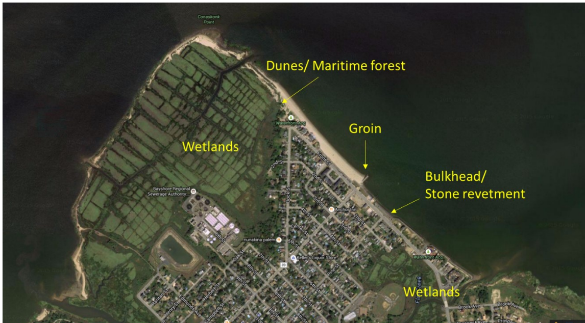
Figure 3.7 Aerial map of Union Beach (500ft) showing location of groin, bulkhead/ stone revetment, beach, dunes, maritime forest and wetlands.
