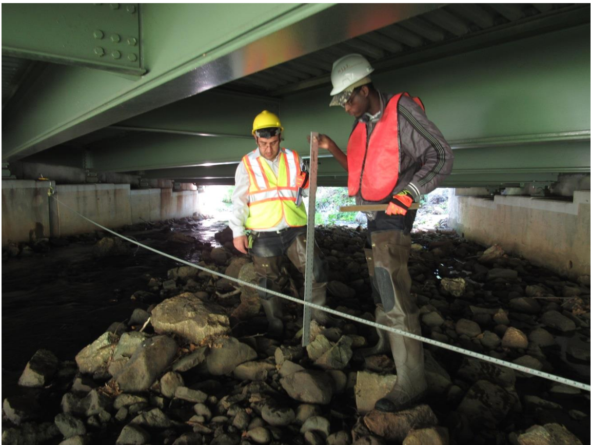
Figure E.16 Bridge # 1605-158 elevation, under the bridge, Wolman Pebble Count section installation and data collection.
