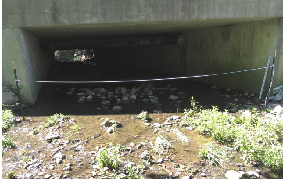
Figure E.2 Bridge # 0709-150 stream-bed sediments close-up and Wolman Pebble Count section installation.
