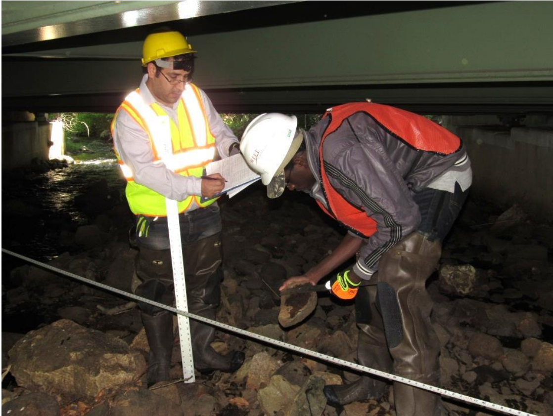
Figure 3.3 Wolman Pebble Count particle selection and measurement.
