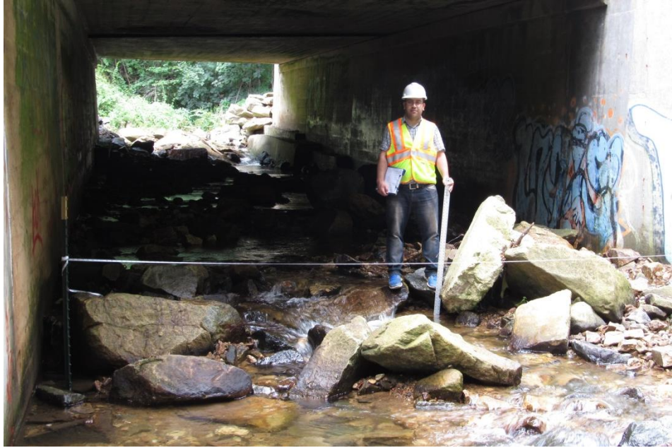
Figure E.20 Bridge # 1417-156 stream-bed sediments close-up and Wolman Pebble Count section installation.
