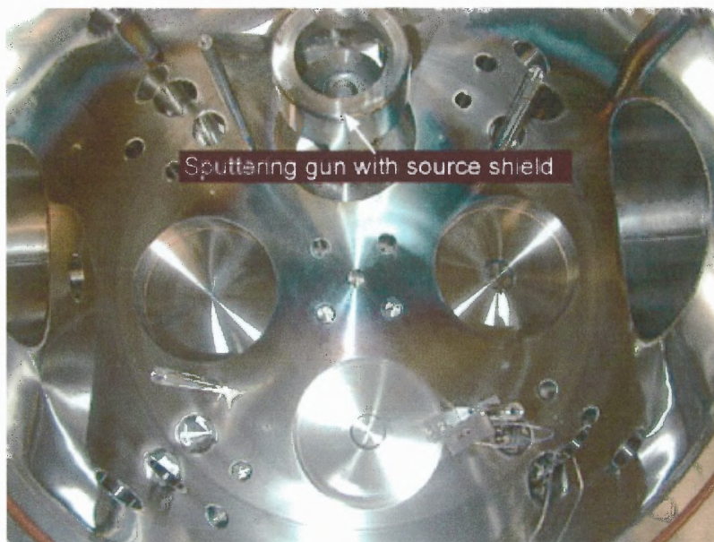
Fig 4.9 Inner view of the deposition chamber showing sputtering gun and source shield.
