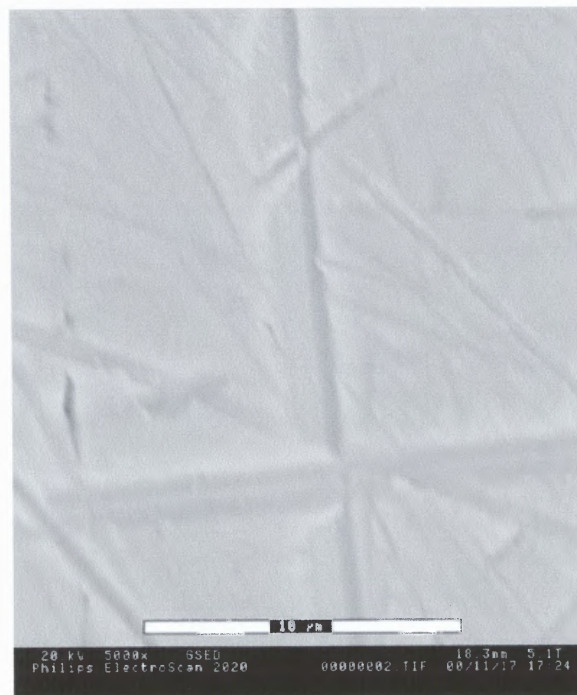
Fig 6.8 SEM image (5000 X) of beta tantalum on steel
