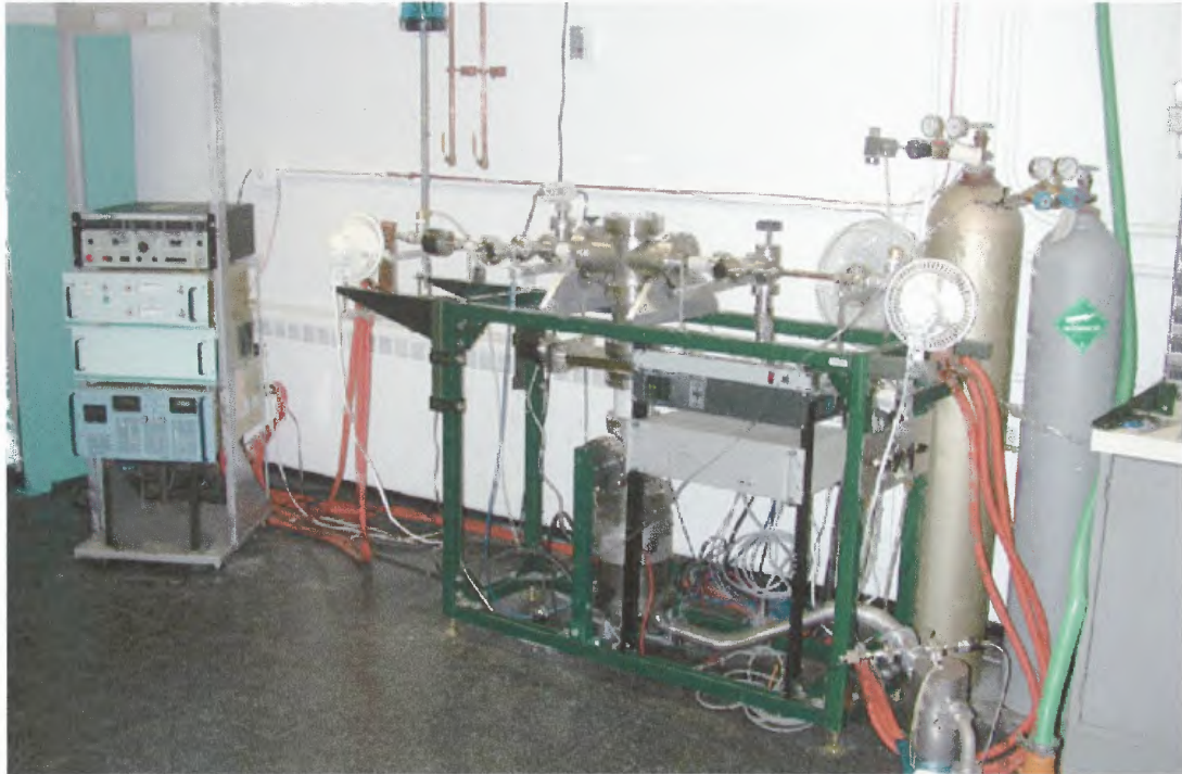
Fig 5.6 Final cylindrical magnetron sputtering system
