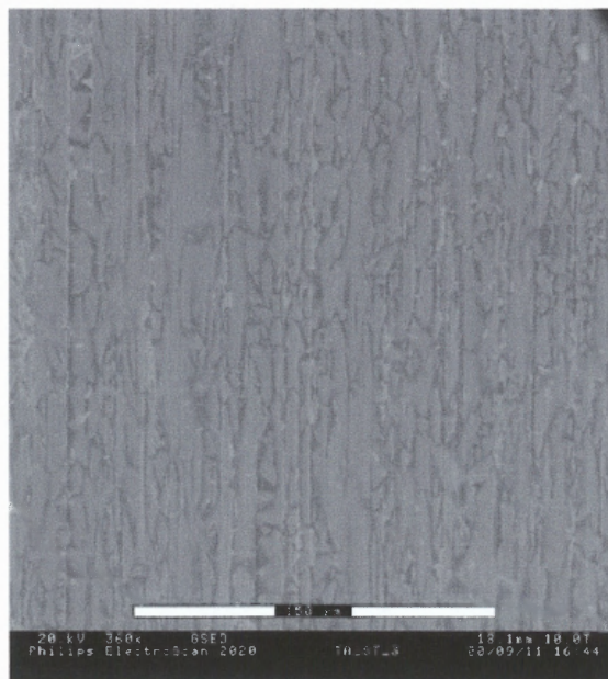
Fig 6.7 SEM image (360X) showing tantalum films deposited along polish lines present on steel surface – film thickness 6000 Å
